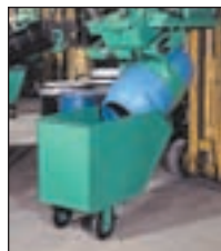
360° rotation on a vertical or horizontal axis; 125° forward tilt.
